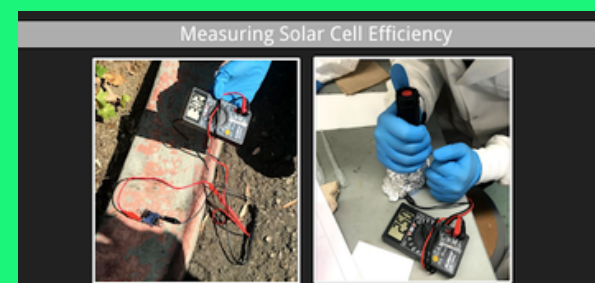
Figure 4: The voltage and the current produced by the solar cells were tested both outside and with LED flashlights using a multimeter. UV Index, temperature, and time of day were kept as consistent as possible.
