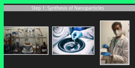
Figure 2: Two types of nanoparticles were synthesized: Gold and Titania. The gold NP were prepared and mixed with a sodium citrate solution and centrifuged to be collected. The Titania NP were prepared using a similar procedure.
