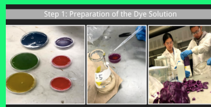
Figure 1: The organic dyes are made by using cabbage juice, a type of anthocynin, which is a dye naturally found in nature. We change its pH levels to achieve the distinct colors using Hydrochloric Acid, Ammonium Hydroxide and deionized water to dilute the cabbage juice.
