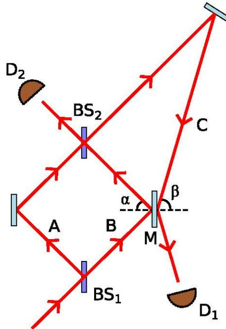
**Figure 2.** Mach–Zehnder interferometer with one output beam reflected back onto the exterior side of mirror M.
