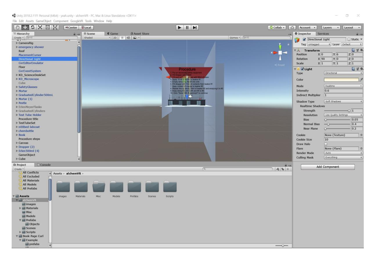
Figure 1. Unity Editor: The following shows our Unity editor, which is our typical work environment for building our simulation. This is essentially where all non-backend work was done, such as scene development, model implementation and other UI elements. This project is divided into four scenes, the main menu, the lab environment, the quiz scene, and the end screen. Most development was done in the lab environment scene.
