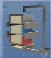
Circulation pump: Recirculates water to encourage biofilm growth. Will not be necessary after growth.
