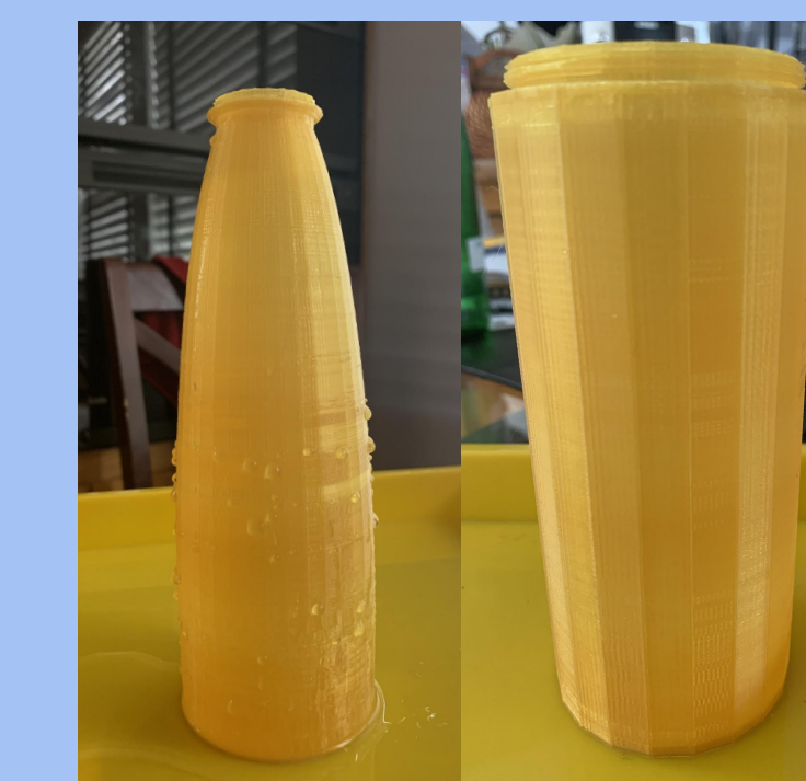
Figure 6: Images of Bottle A and B after the water leakage experiment
