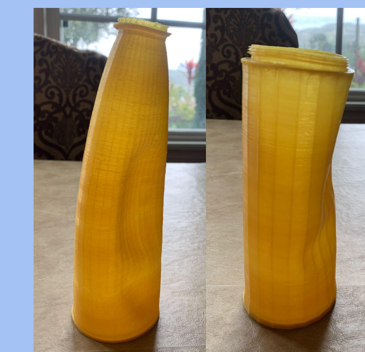
Figure 7: Images of Bottle A and B after the heated water experiment
