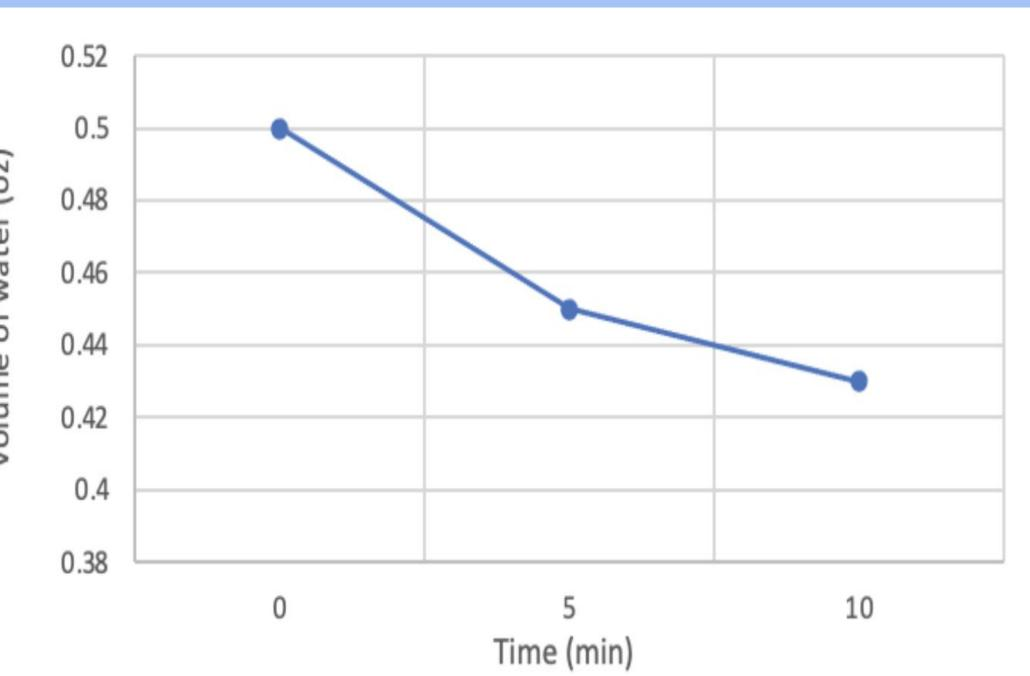
Volume of water evaporated from 1.5 mL pool under fresnel lens in 10 minute time interval
