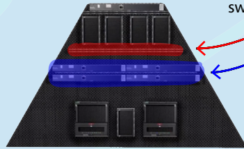
Figure I: Idealized singular trapezoidal computing unit fit with piezoelectric fans, state of the art compute modules and switches
