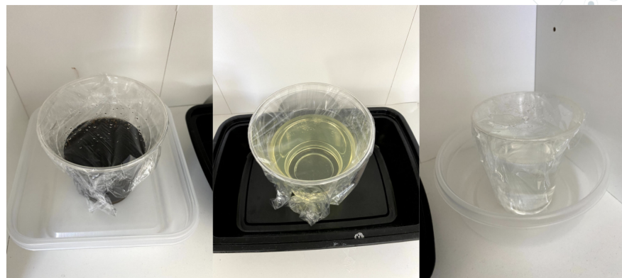
Figure 2: PLA cups with Coca Cola, Bleach and Water. This experiment took place indoors and tested how liquids with varying pH affect PLA.
