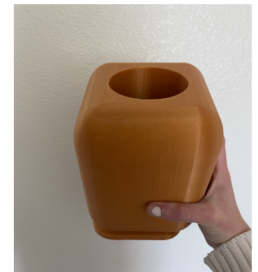
Figure 5: 3D printed PLA water bottle prototype made in makerspace.
