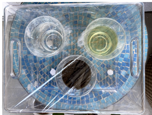
Figure 1: PLA cups with Coca Cola, Bleach and Water. This experiment tested out how pH affects PLA in an outdoor environment.
