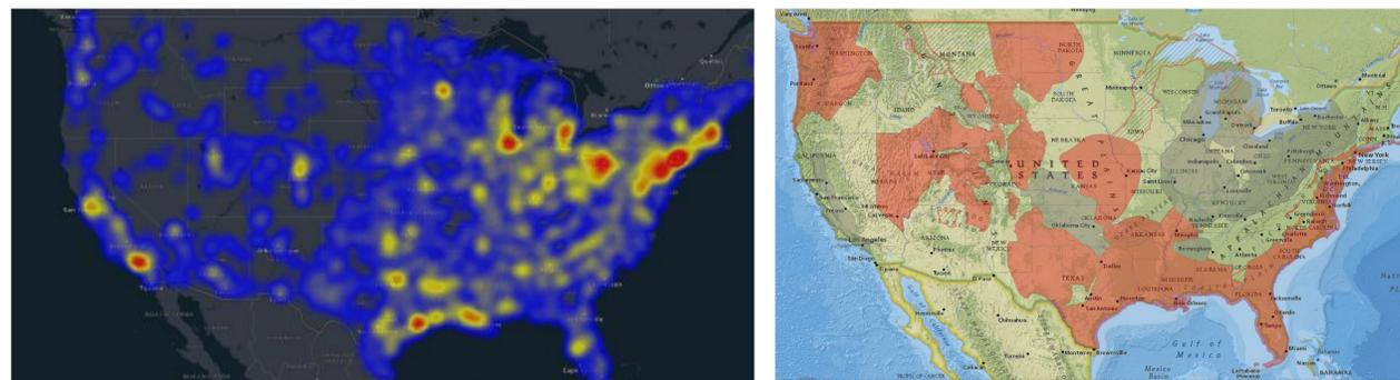
Figure 3: (Left) map of emissions by US ZIP code. Areas in red are high emission zones (Right) Map of porous rock basins (USGS) that can be used/ are being used for Carbon Storage: Appalachian Basin, Atlantic Coastal Plain, US Gulf Coast, Ventura Basin. These regions are identified as ideal for PCC and storage by the USGS, with high emissions and storage potential
