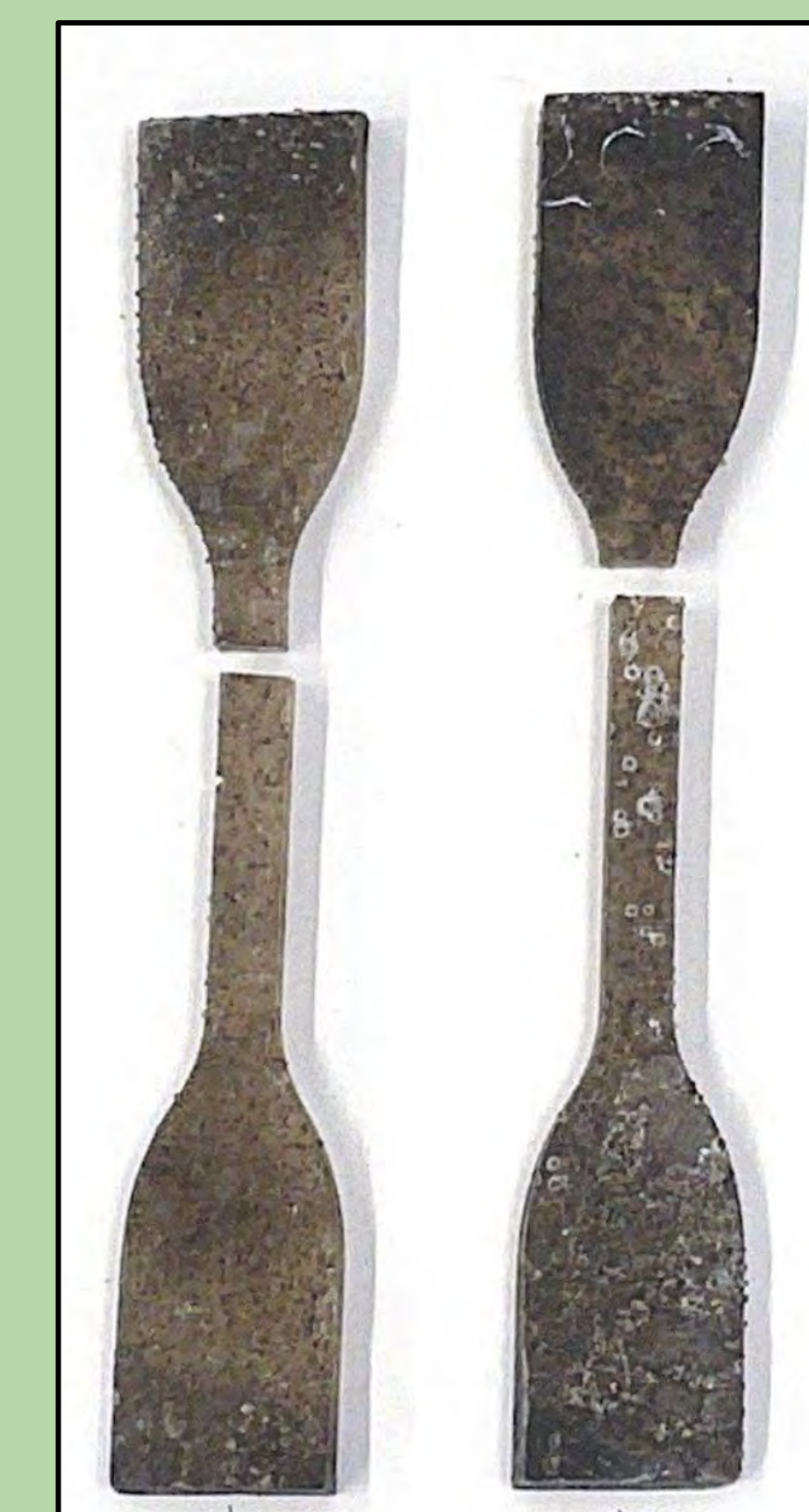
Figure 3b: Breakage points of the 1% coffee dog bones
