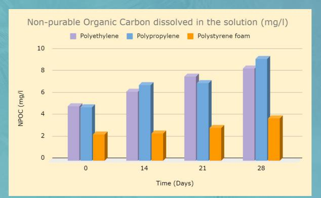
While there was no visible physical change in the plastics, the analysis of the samples demonstrated that a very high amount of Organic Carbon compounds had degraded off the plastic polymers.
